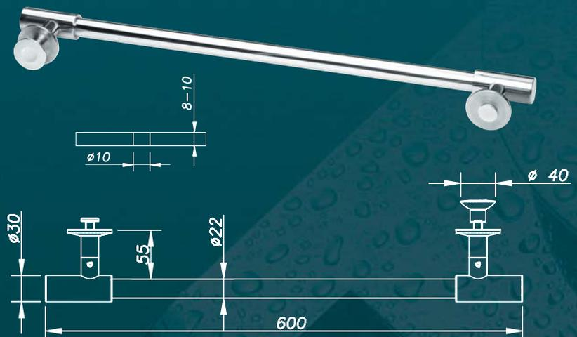
JOINT POUR 8 ET 10mm / SEALING STRIP SAME REFERENCE FOR 8 AND 10mm
